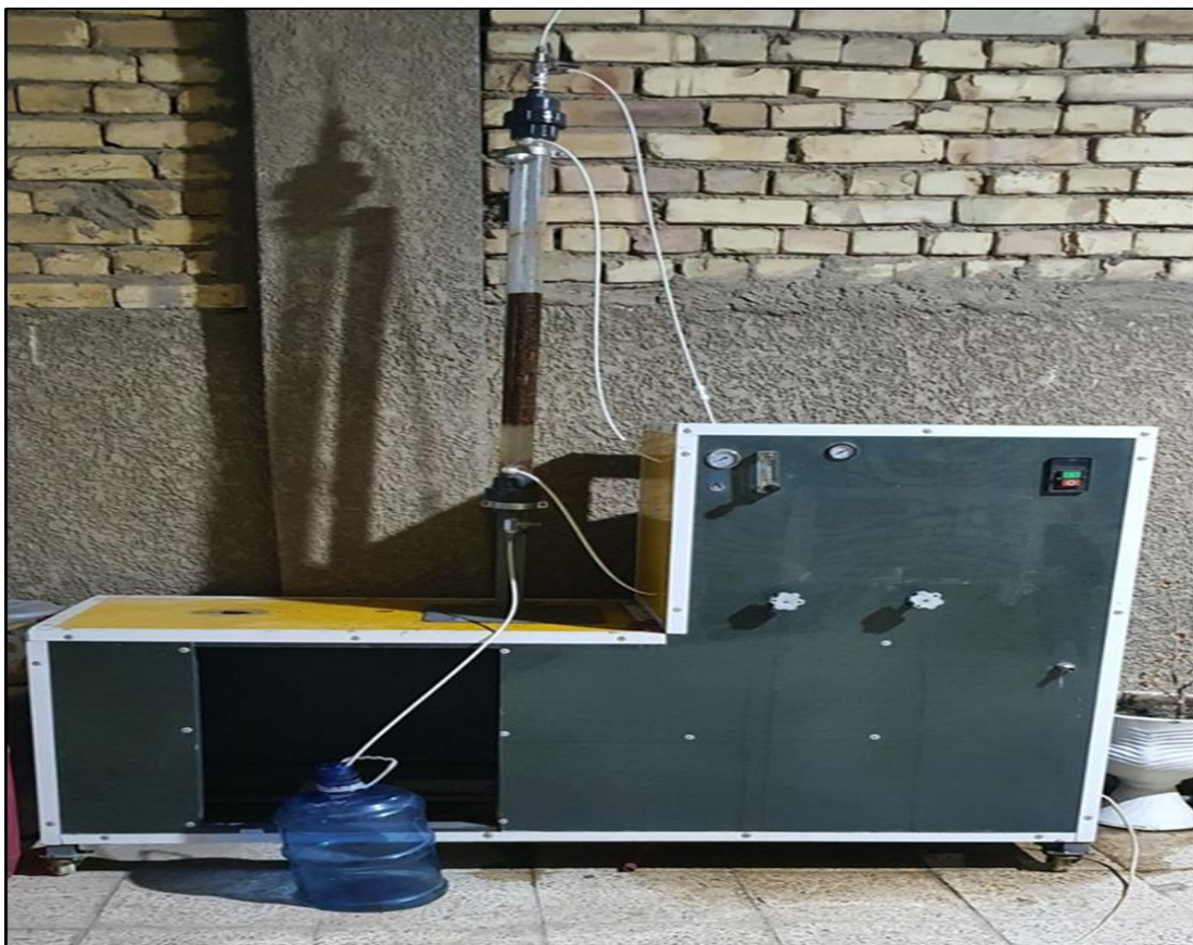
Figure 3.4: Photograph of the inverse fluidization bed Unit
